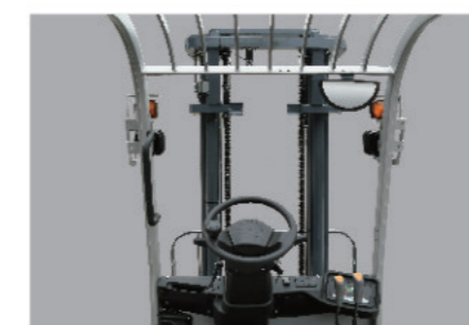
The mast with large opening offers good driving vision ensuring operation comfort and safety.
