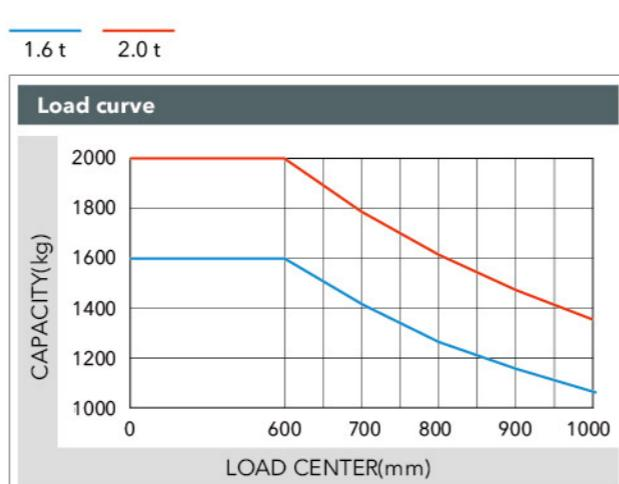
**Note:** The vertical axis denotes capacity and the horizontal axis denotes load center, which is calculated from front face of fork to centre of load. Standard load is one cubic metre hence 500mm load centre. When tilting forward or using non-standard forks, the capacity will be reduced as load centre is increased.
