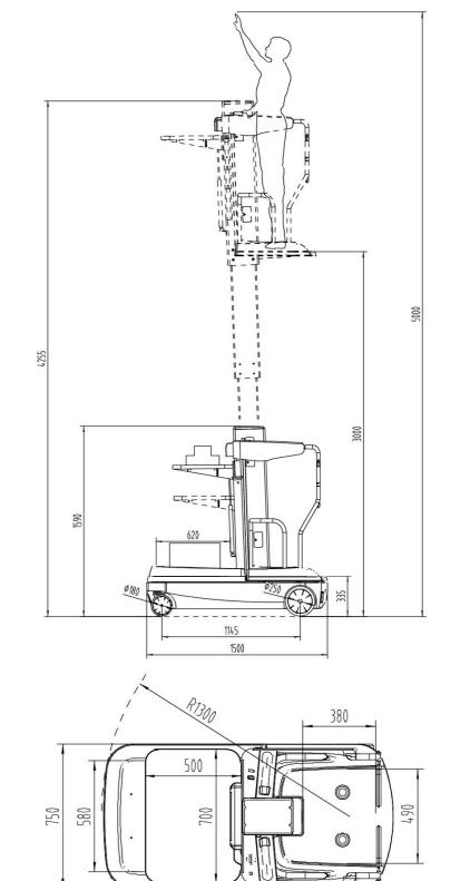
The picking height can reach to 5m, easy for picking-up or storage of items at 3rd rack level, sprice tag exchanged or ceiling upholster and light fixing.
